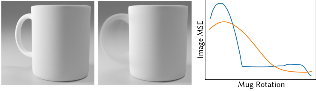
Figure 1.2: An exemplary visualization of an inverse rendering problem with a plateau, and our solution. In a rigid optimization, rotating the cup around its z -axis introduces a plateau in the cost landscape (the blue curve) as soon as the handle is occluded by the cup. In our formulation (middle image), the smoothed cup’s handle always is (slightly) visible and hence continuously influences the objective, leading to the much smoother orange curve.
