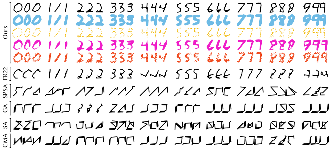
Figure 5.12: We sample the latent space of our trained variational auto-encoder (VAE) and show a variety of style transformations (rows), enabled by the spline formulation, on three digits per MNIST class. The first row displays the output of the spline renderer on which the surrogate operates.
