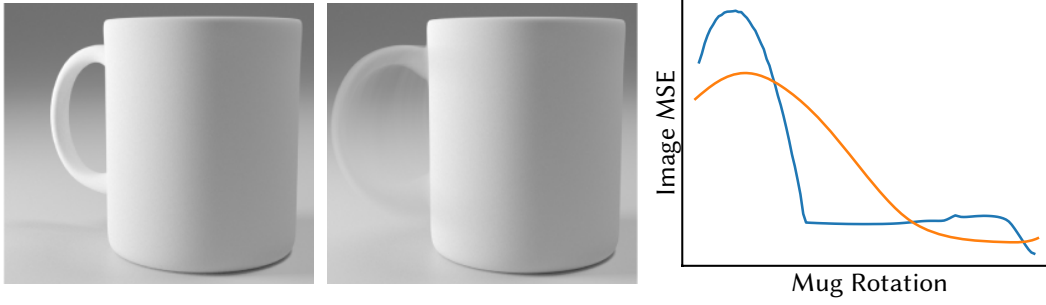
Figure 4.3: Optimizing the cup’s rotation in the hard (left, blue) and smooth (right, orange) setting (note the blurred handle). The image-space loss landscape is displayed on the right: blurring resolves the plateau.
